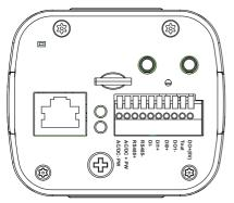
The day/night mode DI connection enables the synchronization of IR light and the automated day/night switching mechanism on the camera.
