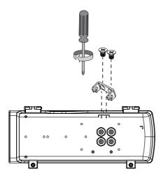
**15.** Install the housing to the wall-mount bracket by aiming and pressing the spring mortise, and hook the bracket onto the groove in the spring mortise.
