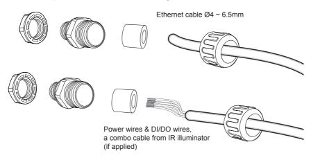
You may need to remove the RJ45 connector, and use a crimping tool to connect the Ethernet wires to an RJ45 connector inside the enclosure. Use an Ethernet cable of the width of  $4 \sim 6.5$ mm.
