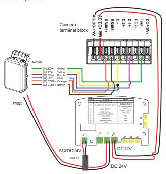
**13.** You can connect the ground wires together and connect them to the DI- ground pin on the terminal. Use a small flat blade screwdriver to press the lever on the terminal block.
