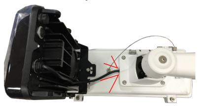
16. Secure the housing to the bracket by fastening 4 T30 screws.
