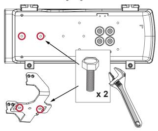
3. Secure the U bracket to the IR illuminator using the included hex screws.
