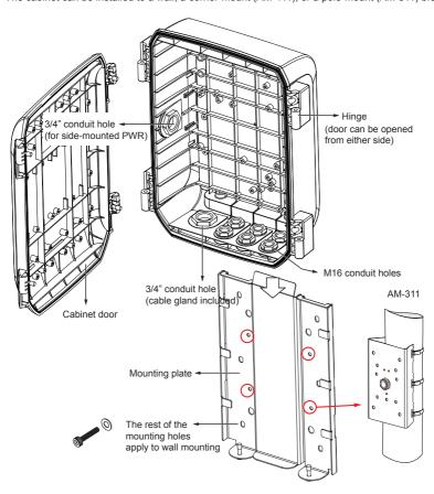
You can use the unused mouting holes for installing several cable clamps for routing the cables.
