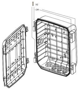
Pass the Ethernet and I/O combo cables through the M20 cable glands, and into the cabinet. You may need to open the cabinet. Secure the camera mount bracket (here a speed dome bracket is shown) to the cabinet. You can then install the camera. Refer the camera's documentation for information.
