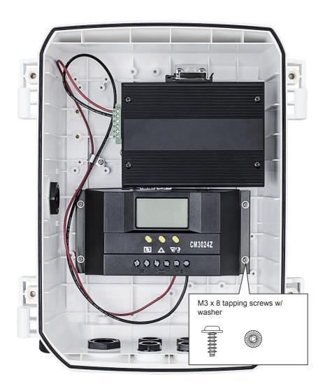
Insatll 3/4" and M16 cable glands and cable conduits to protect the cables and the wiring to the outside of the cabinet. Properly install the cable glands so that the product's IP rating is maintained. If not properly installed, water may seep into the cabinet, causing damage to devices inside.
